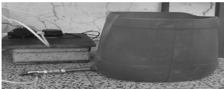
Figure (4): Raw water collection tank
