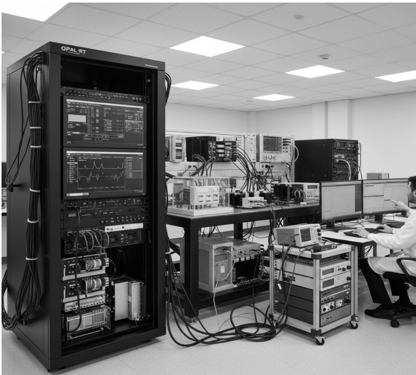
Fig. 6. A real-time digital simulator (e.g., OPAL-RT), used in advanced power systems labs for HIL validation.
