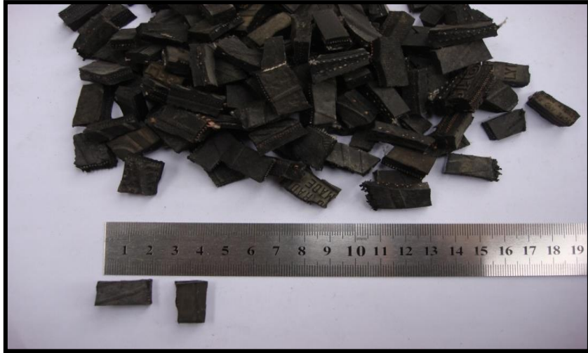
Figure (1): Tire rubber fibers (length = 20 mm)
