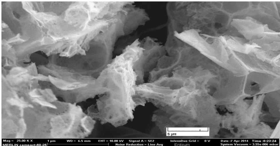
Figure (10B): Erbium oxide particles Shows an even distribution in SEM (2500KX).
