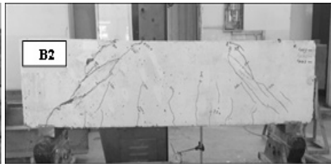
Plate 5. Crack Pattern for Beam B2 after Testing.
